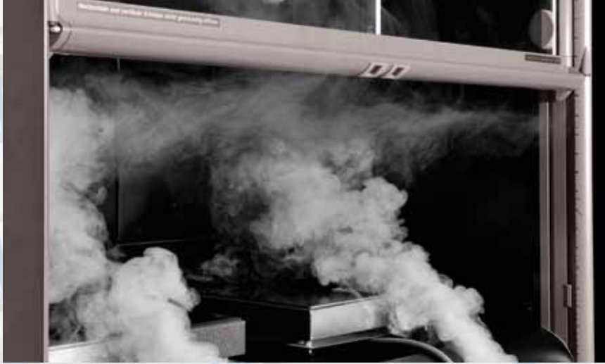
Standard fume cupboard with heating source
